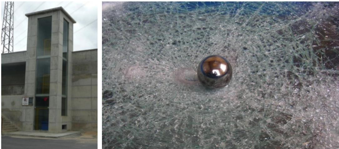
Figure 10: Test tower for 9m high hard body drop and glass specimen broken but not perforated after hard body drop test.
