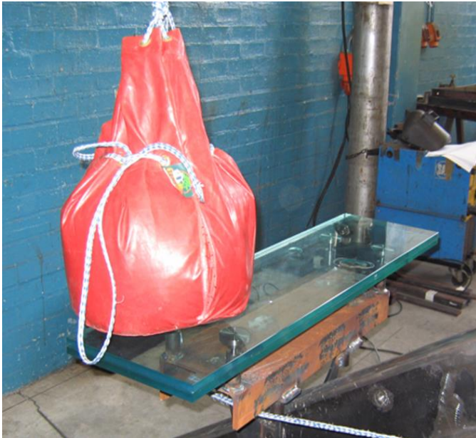
Figure 6: Glass Floor load testing
