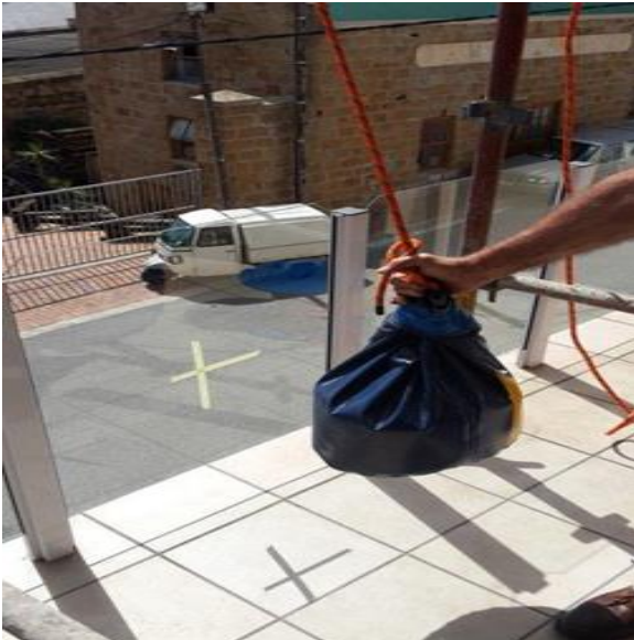
Figure 13: Original old balustrade impact test
